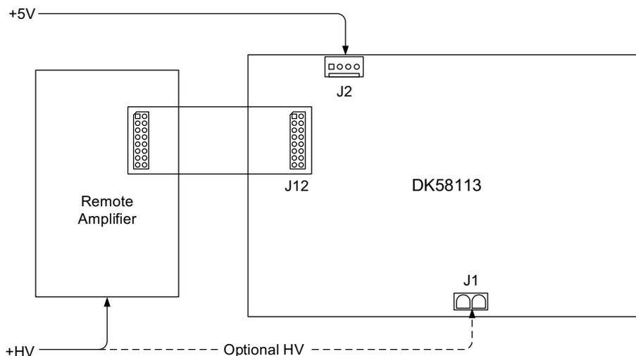
In addition to the DK58113's on-card switching amplifier, J12 provides connections for an external remote switching amplifier. This connector is typically used to interface with user-designed amplifiers that service higher power motors, or motor or actuators that require a special bridge configuration. Such an external amplifier connection is shown in Figure 2-7.
