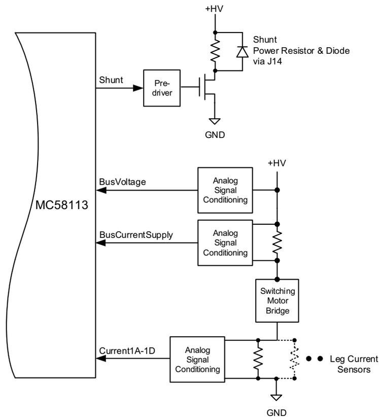
Figure 2-6 shows the DC bus monitoring circuitry used with the DK58113 board. This circuitry is designed to work with the MC58113's DC bus management and protection logic. These functions include overcurrent protection, over and under voltage detection, ground fault detection, and shunt resistor control.
