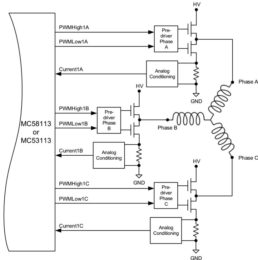
As shown in the table below six PWM output signals and three analog feedback signals interface between the MC58113 IC and the DK58113's switching amplifier.
