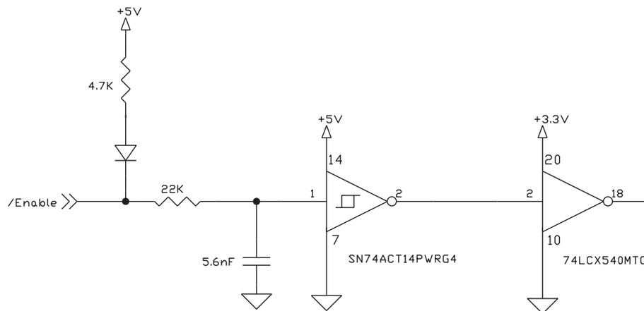
The output driver for FaultOut is shown in Figure 2-15. This circuit can continuously sink over 100 mA and source 4mA from a pull-up resistor to 5V. The diode in series with the pull-up resistor allows loads powered from up to 24 VDC to be switched. The FET driver is internally protected from shorts up to 30 V.
