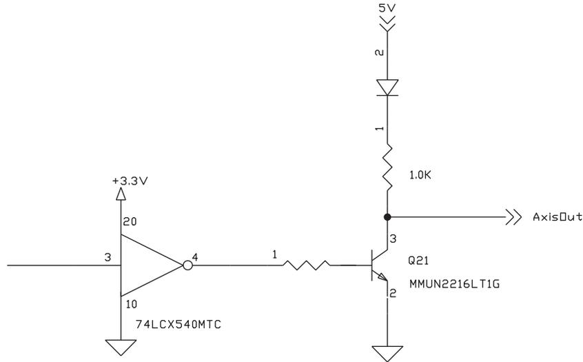
AxisIn and AxisOut are versatile I/O signals. They are not dedicated to any particular motion control function but can be programmed to implement a wide array of system integration functions. See the *Magellan Motion Control IC User's Guide* for more information on configuring and programming these signals.
