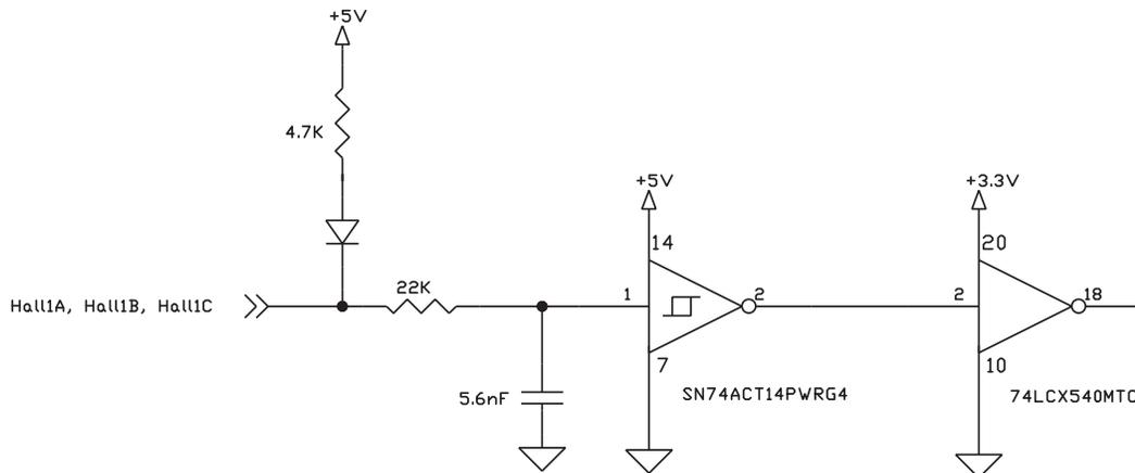
The Hall signals are only used with Brushless DC motors. They are used to directly commutate the motor in 6-step commutation mode or to provide an absolute phase reference for sinusoidal commutation.
