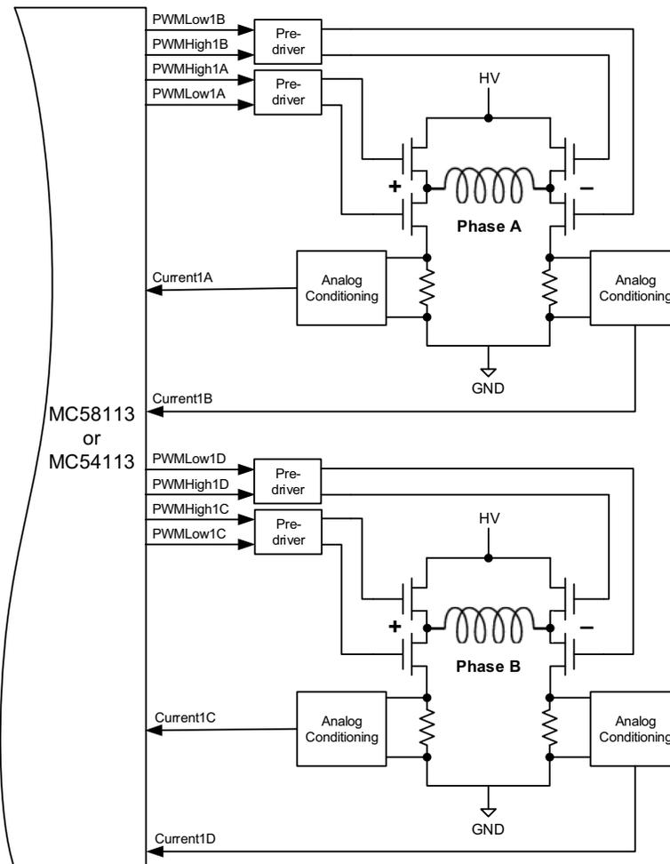
As shown in the table below eight PWM output signals and four analog feedback signals interface between the MC58113 IC and the DK58113's switching amplifier.
