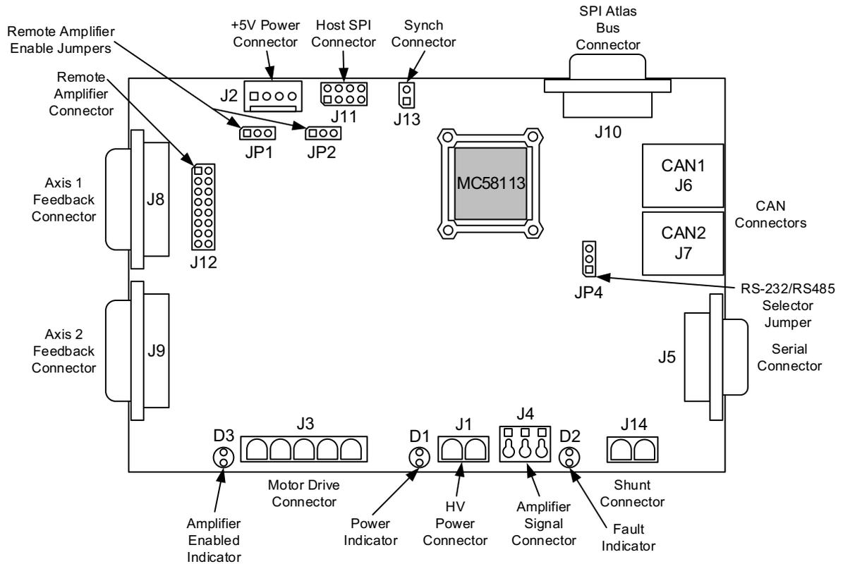
There are 14 user-accessible connectors on the DK58113 card. See Figure 3-1 for the specific locations of the connectors on the card. The connectors and their functions are outlined in the following table:
