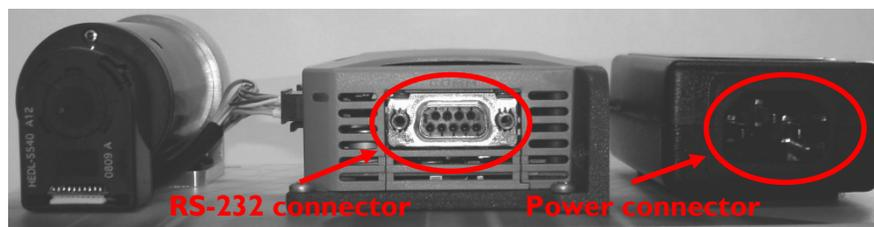
Figure I-1: ION Demo Kit - rear view
