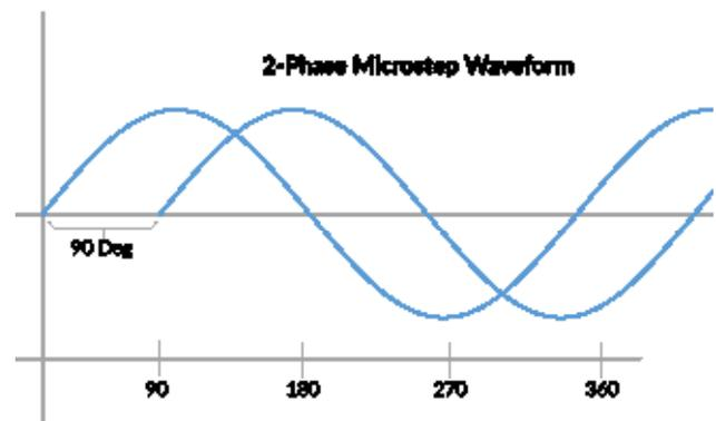
Figure 1: 2-Phase Microstep Waveform
