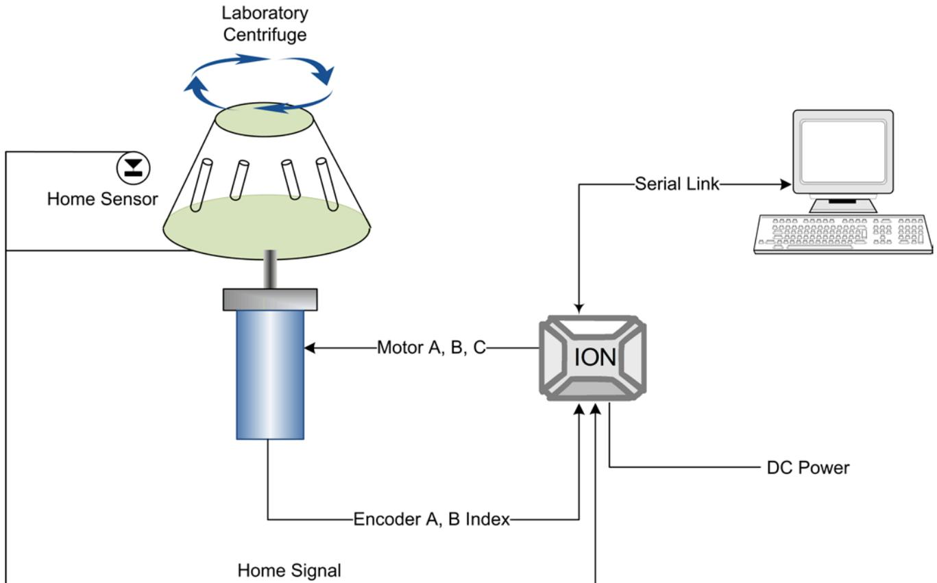
The figure above shows an ION Digital Drive, which contains a single-axis motion controller and amplifier, driving the centrifuge. The centrifuge provides quadrature A, B, and Index signals, and a home signal is input to the ION to reference the axis after power up.
